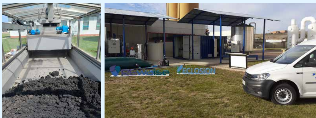
On the left, sludge dried using a solar system. On the right, End-to-end Water Cycle Innovation Centre at the Salamanca WWTP.
