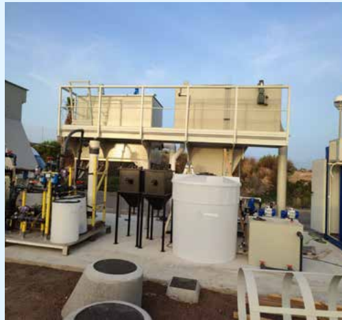
From right to left, ballasted clarification (CLARIFAST) and dissolved air and/or ozone flotation (DAFAST).
